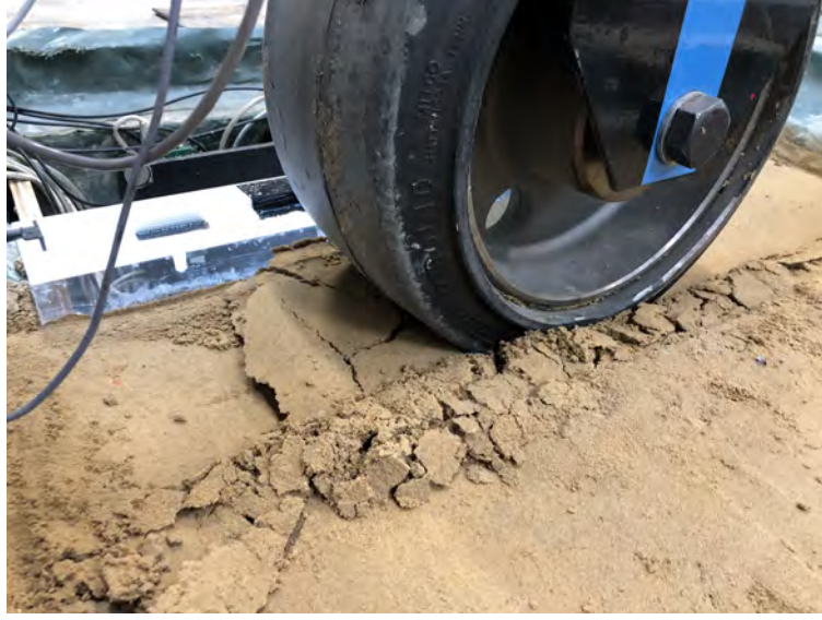
Figure 23: Formation of soil pile in front of the wheel
