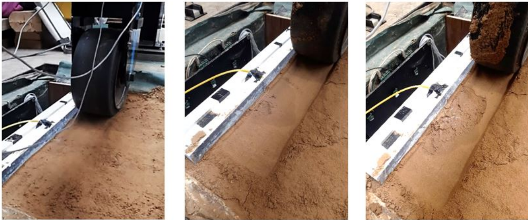
Figure 26: Pothole forming after 2 cycles on wet subgrade
