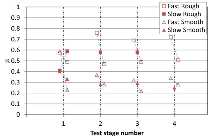
Figure 8. SNS summary results showing initial peak and residual interface friction values.
