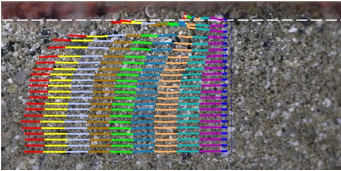
Figure 9. PIV analysis of sieved GOG sample at the start of shearing; showing shear zone of approximately 2mm thickness.
