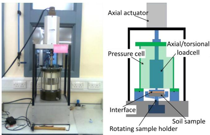
Figure 1. Photograph and schematic diagram of the Cam-Tor machine.
