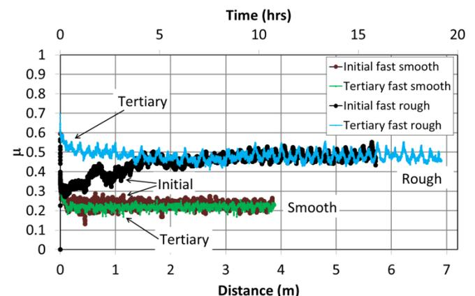
Figure 11. Comparison of initial and tertiary GOG test stages for rough and smooth interfaces.
