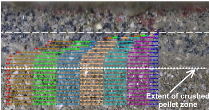
Figure 10. PIV analysis (sieved GOG sample) of the end of shearing showing shear zone of approximately 1mm thickness and extent of CPZ.
