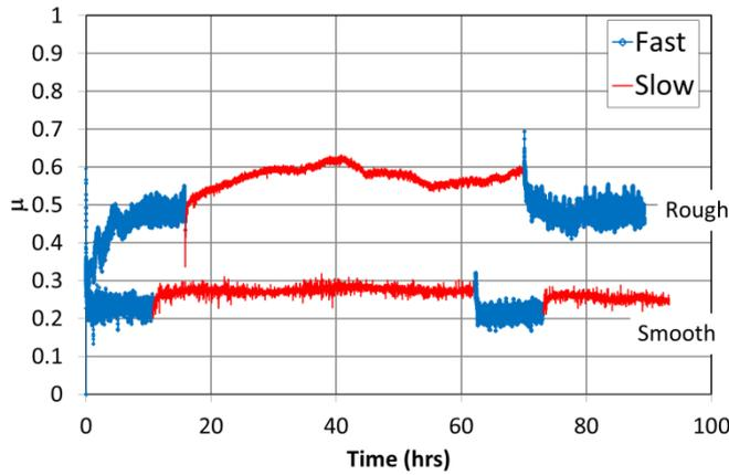
Figure 6. Example rough and smooth interface tests for GOG sample.
