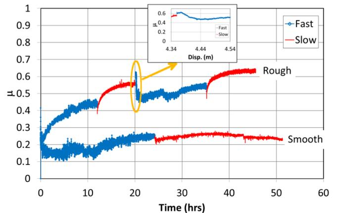
Figure 5. Example rough and smooth interface tests for SNS sample. Inset: initial fast peak plotted on semi-log axes.
