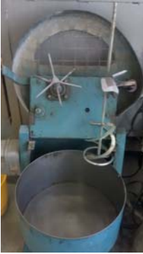
Figure 27: The pan-type mixer used in earlier batches. This pan was also used with the pictured drill-mounted 'whisk' attachment.
