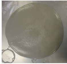
Figure 10: The result of a slump-flow test: a circular disk of material.
