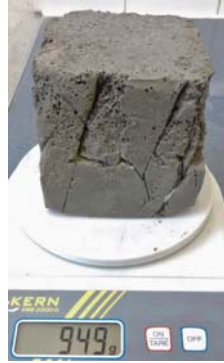
Figure 28: A poor-quality cube from an early mix attempt. Note over-density, segregation (larger bubbles visible closer to the top), crevices and rounded corners due to intruding 'cling film'.
