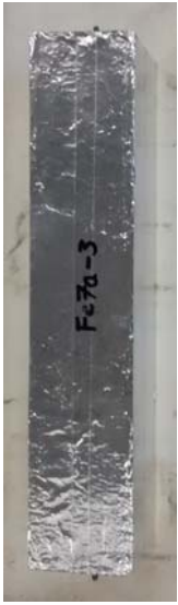
Figure 11: A shrinkage prism covered in foil tape. Note the protruding end pins.
