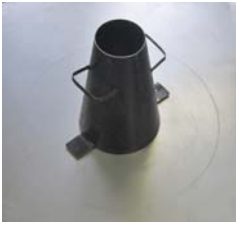
Figure 9: The slump cone and base plate used for the slump-flow test. Note the inscribed circle for measuring t_{500} time.
