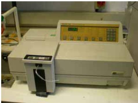
**Figure 12 (left):** Unicam 8620 UV/Visible Spectrophotometer
