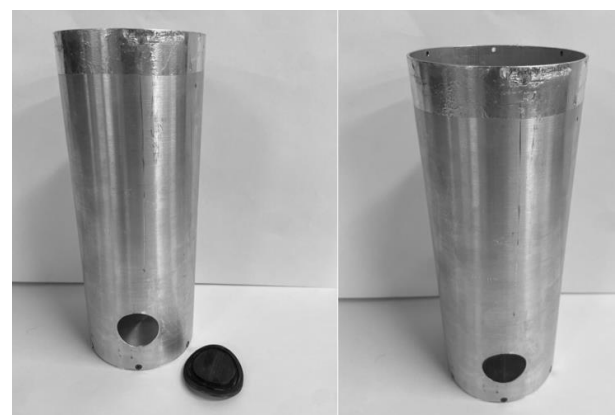
Figure 1. Model shaft lining with an opening
