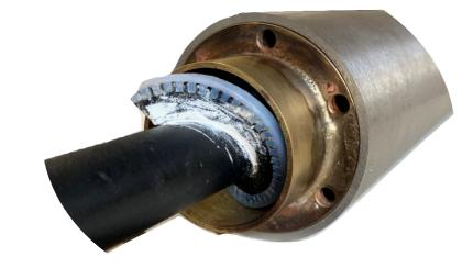
**Drive system:** the mini-TBM will be driven forwards by an actuator, and a motor will rotate the auger and cutterhead. The mini-TBM will be used in a series of centrifuge tests in sand and clay, comprising a parametric study. Tests will be at 50g, replicating a tunnel with a diameter of just under 4m
